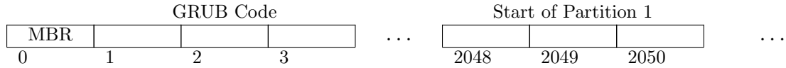
Figure 2.3: Layout of the disk image we will create for the GRUB hello world.
