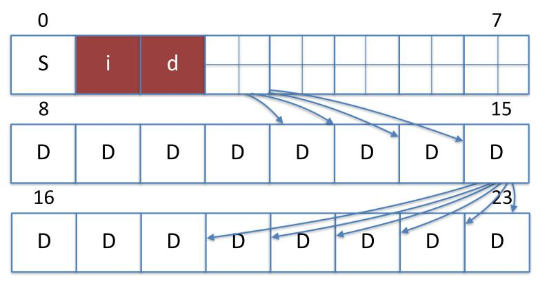
If an inode can only point to 4 data blocks, max file size is 16 kbytes (4 \* 4k).
