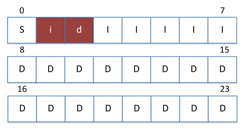
Superblock tells us parameters of the filesystem like how many inode blocks and data blocks there are and where to find the root inode.
